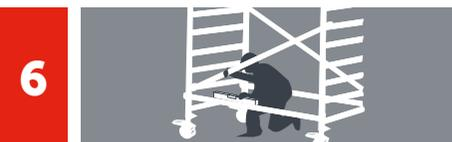
Afterwards, the leveling of the base (both in the horizontal and vertical planes) must be checked in the place where the tower will be used. Using a spirit level, make sure that the lateral frames stand upright and the horizontal braces are properly assembled. Any due corrections will be performed using the leg adjusters.
