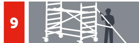
Assemble the outriggers. These must be tied to each corner of the tower in the same tube we have inserted the legs, by using the incorporated clamps. The upper clamp must be fixed just below a joint of the lateral frame in order to avoid any slipping. Make sure that the revolving brake shoes are firmly in contact with the ground. Assemble the outriggers or stabilizer bars as described on page 11 in this guide.
