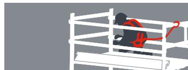
ALUFASE recommends installing toe boards on every work level. Make sure that the platform windlocks on all the platforms have been set. Before using the scaffolding, check that the locking casters are activated and the outriggers are assembled correctly. Go through the checklist attached to this guide, before using the tower.
