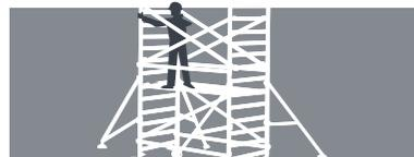
In the Model 400, place an inner access ladder only if there is not a built-in ladder on the lateral frame itself. Place another platform at the top and repeat step number 10 for every additional module. Structurally, platforms cannot be spaced out for intervals of more than 13' (4 m). However, ALUFASE recommends keeping 6'6" (2 m) as the maximum distance between platforms.
