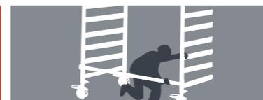
Place another lateral frame on the opposite side and insert the free end of the horizontal brace at the same height (generally at the base). When assembling towers with a double width (4'5" / 135 cm), place two horizontal braces at the base (one on each side of the lateral frame).
