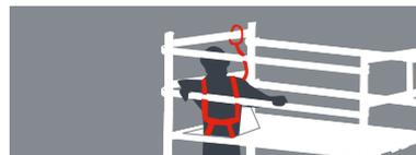
Assemble, on the lateral guardrail frames, two horizontal braces on each side of the tower (the upper hook resting on the flanges off the guardrail frame in order to avoid slipping), thus sealing off the working level completely. NOTE: Remember that the correct position for the braces is with their hooks facing outwards.
