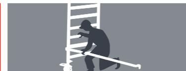
Insert the end of a horizontal brace (with the hooks facing out) into the lower part of a vertical tube and place the other end of the brace on the ground (to hold the structure).
