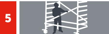
Assemble two diagonal braces opposite one another. The hooks of the braces must be fitted in the rungs of the lateral frames (generally, on the 2<sup>nd</sup> and the 5<sup>th</sup> rung) and as close as possible to the vertical tubes of each lateral frame. When assembling towers with a double width (4'5" / 135 cm), 4 diagonal braces are required, placing 2 on each end of the lateral frames in the shape of an x.
