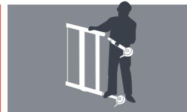
Introduce the caster/base plate into the adjustable legs and insert these into the bottom holes of the two lateral frames. To level the towers out, spin the leg adjuster around the threaded leg until an adequate leveling is achieved (check with the spirit level).
