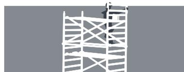
Once the top level has been placed, and always using the safety harness, assemble the guardrail frames and insert all the metallic interlock clips. Never assemble platforms on top of the guardrail frames of the scaffolding. Keep yourself secured (use a double point of anchorage if necessary).
